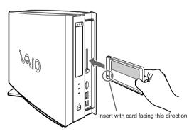
When the card is inserted correctly, the eject button pops out. If the card does not insert easily, make sure the card is not being inserted upside-down or backwards before carefully reinserting the card into the slot. Do not forcibly insert the card.
